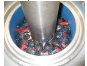
Ram BOP – Front Packers, Top Seals & Door Seal Function Pressure Test
