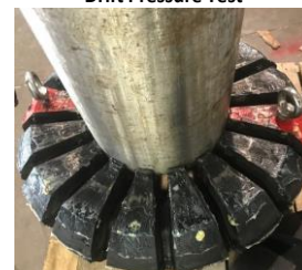
Annular BOP – Packing Element Drift Pressure Test
