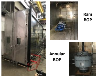
Temperature & Pressure Cryogenic Test Chamber
