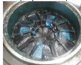
Annular BOP – Packing Element Drift Pressure Test
