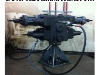
Ram BOP – Front Packers, Top Seals & Door Seal Function Pressure Test
