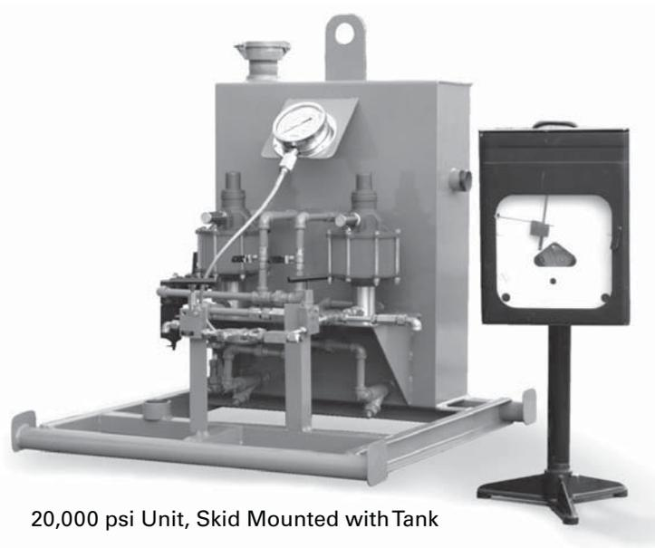
20,000 psi Unit, Skid Mounted with Tank
