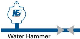
Surges in fluid systems caused as a result of sudden valve closures, pump shut-downs or start-ups, can lead to pressure build-ups that are large enough to rupture piping, piping supports and damage downstream equipment. This phenomenon, also known as water hammer, results from the sudden change of kinetic energy (of the flowing fluid) to pressure energy.
