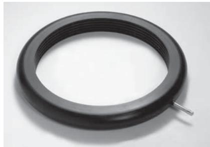
Mud Tank Union Air Tubes are molded from Nitrile Rubber. The use of Union Tubes allows quick installation of plain end pipe between mud pumps and tanks. They also assist in absorbing pulsations.
