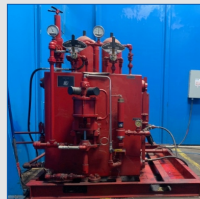
BOP Test Unit Hydraulics
