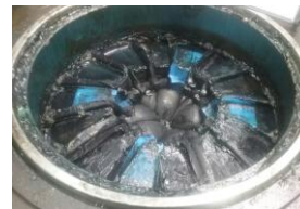
Annular BOP – Packing Element Drift Pressure Test
