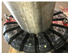
Annular BOP – Packing Element Drift Pressure Test
