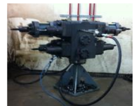
Ram BOP – Front Packer, Top Seal & Door Seal Function Pressure Test
