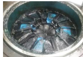
Annular BOP – Packing Element Drift Pressure Test
