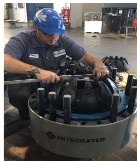
Annular BOP Inspection & Seal Replacement
