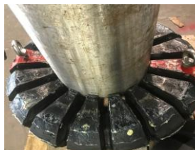
Annular BOP – Packing Element Drift Pressure Test
