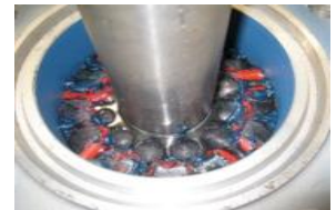
Ram BOP – Front Packer, Top Seal & Door Seal Function Pressure Test
